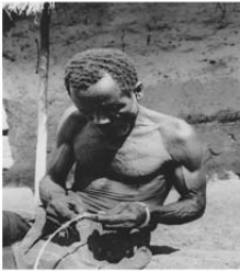
Manufacture of the Mutuga, village of Ngaba. First (left): preparation of the supple fiber (vegetable and animal hair) core; second (above): rolling of the wire in tight coils on this core. 1956, Katanga, DRC. HPI 1984.25.69-28 and HPI 1984.25.69-25, collection RMCA Tervuren; photo LPHMK, 1957, RMCA Tervuren © Graphic L.G.-Marot
