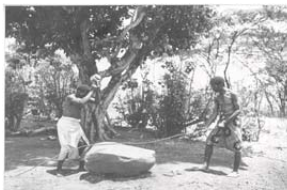
Pounding of the copper ingot into an irregular bar (the Museya ) about 3 metres long. Village of Nguba, 1956, Katanga, DRC. HPI 1984.25.69-30, collection RMCA Tervuren; photo UMHK, 1957, RMCA Tervuren © Graphic L. G.-Marot
