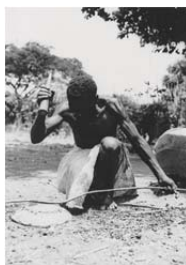
Beating the bar (the Museya ) to regularize and elongate it. Village of Nguba, 1956, Katanga, DRC. HPI 1984.25.69-34, collection RMCA Tervuren; photo UMHK, 1957, RMCA Tervuren © Graphic L. G.-Marot
