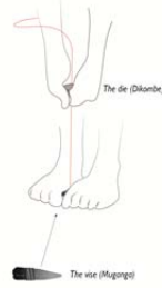
Setting the wire and the die for drawing the Nsambo. Village of Ngaba, 1956. Katanga, DRC. HPI 1984.25.69-26, collection RMCA Tervuren; photo LPHMK, 1957, RMCA Tervuren © Graphic L.G.-Marot
